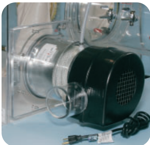
#800-HEPA/S and #800-HEPA/S/EXP for export models (External view with exhaust outlet connector)
