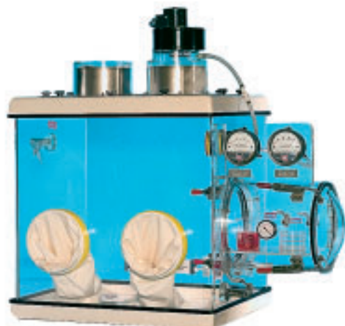
#800-HEPA/D. Open exhaust (double) HEPA filtration system
